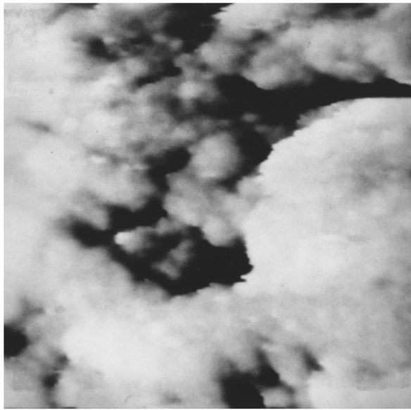
FIG. 1. STM image of nc -Si:H. The scale is 50 nm×50 nm.
