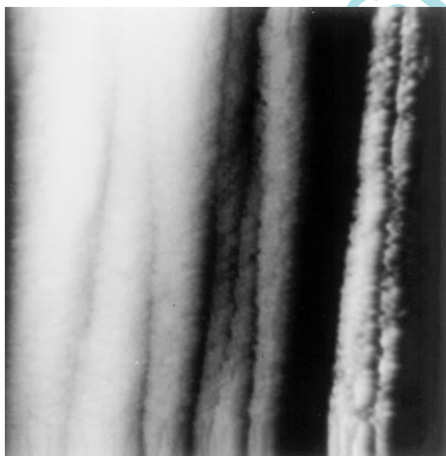
FIG. 2. STM image of PAN-based carbon fibers without treatment on submicron scale. (1200 nm × 1200 nm)
