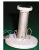
Fig. 5. Tube scanner structure in sample-scanning AFM
