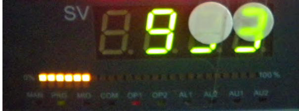
Fig. 1. Photograph illustrating the transparency of pure KNLTN (left) and KNLTN-La 0.01 (right) ceramics.
