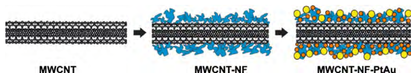
Scheme 1. Stepwise fabrication of f -MWCNTs–NF–PtAu composite film.
