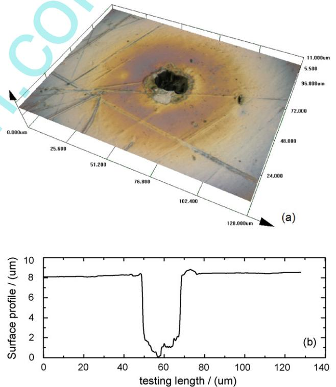
Fig. 2. Surface profile of the erosion pit with ring are tested by confocal laser scanning microscope. (a) Picture of the pits scattered on the surface and (b) surface profile of the cross section of the pit.
