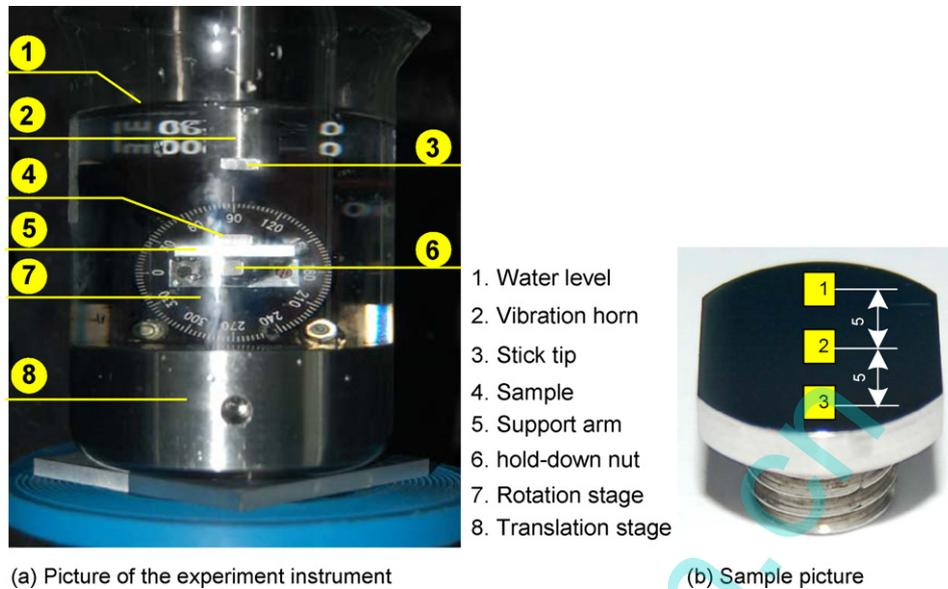
Fig. 1. (a) Vibration cavitation system, and (b) the picture of the sample with testing regions.
